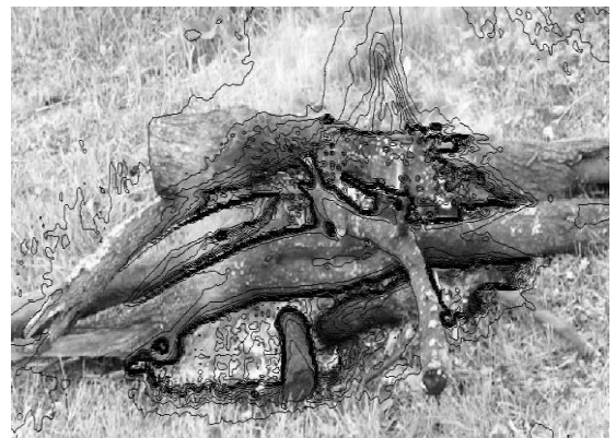
Figure 9. The lines of the indicating the temperature from 1000 to 10000 shown over the color image. Note: original image is in color.
