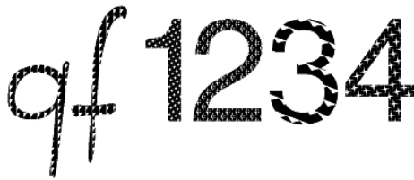
Figure 6. Different raster elements on each letter, with variation in liniature and angle
