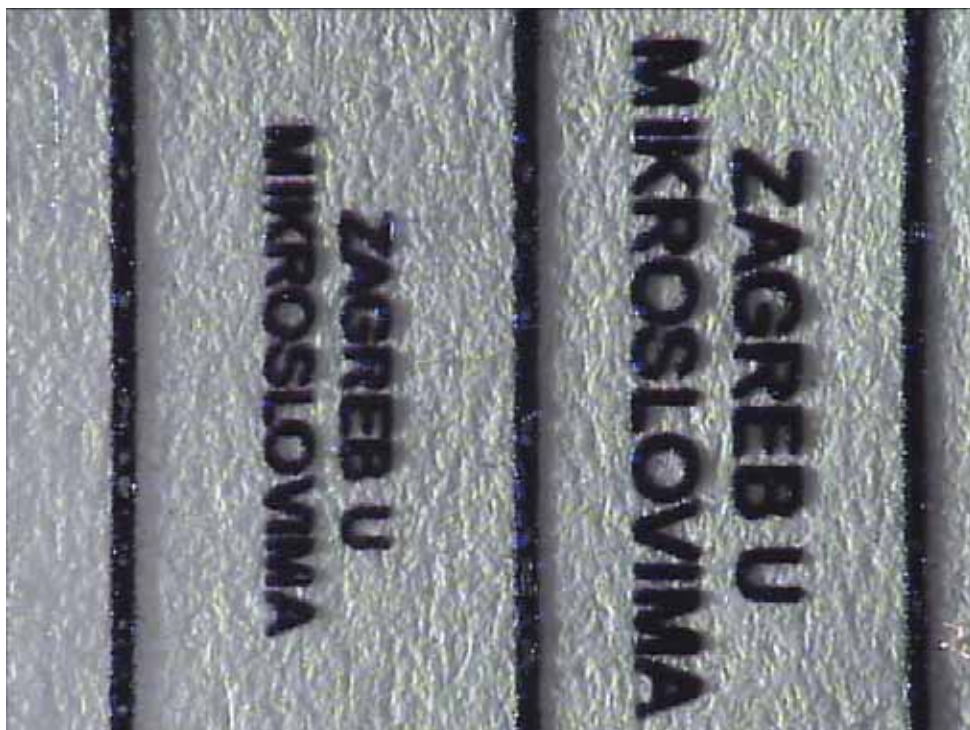
Figure 2: Proposal for a tactile structure design, Xeikon digital print
