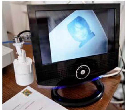
Detection of hidden image in the near-infrared (NIR) of the output from printer with NIR apparatus (part of the system)
