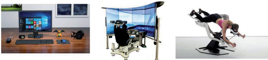
Figure 2: a) non-immersive system b) semi-immersive system c) fully-immersive system (Google images)
